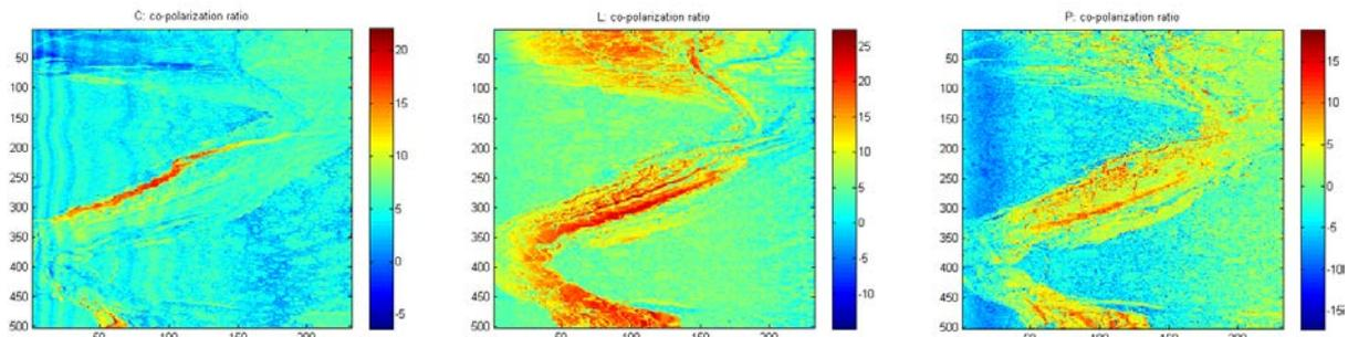
Figure 8 AIRSAR co-polarization ratios (VV/HH). C-, L- and P- band. Scene: 6830. Legends in dB.
