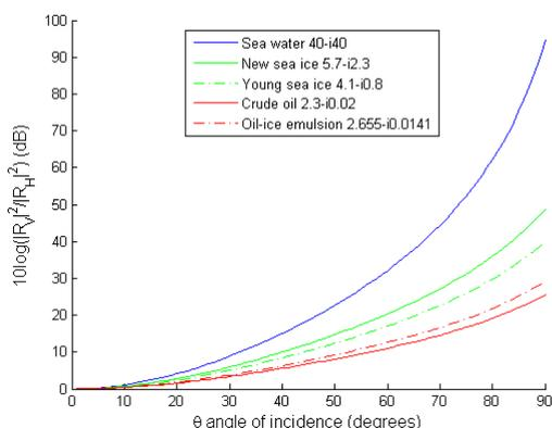
Figure 5 Co-polarization ratios for various representative dielectric media, primarily at 10 GHz. The dielectric properties for sea water are valid for  $S=35\%$ ,  $T=0^\circ\text{C}$  [11]. The dielectric property of crude oil is from [12]; the dielectric property for oil-in-sea-ice 50/50 emulsion is derived for  $-2^\circ\text{C}$  from the linear mixture model in section 2.4; and the sea ice values are from [6].
