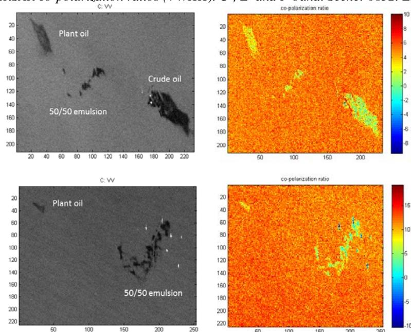
Figure 10 Left: VV channels. Right: Co-polarization ratios (VV/HH) and legend in dB. Wind speed 1 m/s (top) and 6 m/s (bottom). RADARSAT-2 Data and Products© MDA LTD. (2011) - All Rights Reserved.
