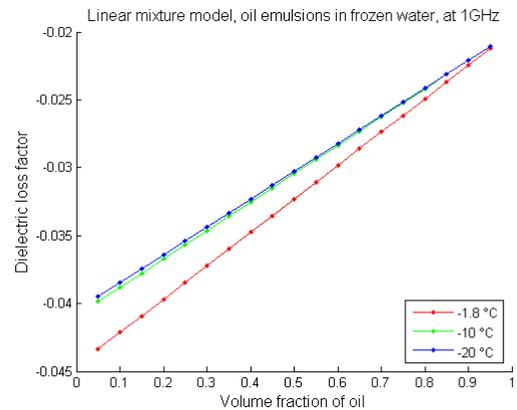
Figure 2 Dielectric loss factor for oil emulsions in frozen water at 1 GHz.
