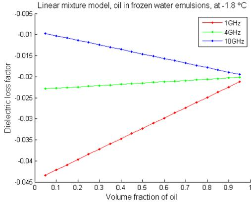
Figure 4 Dielectric loss factor for oil emulsions in frozen water at  $-1.8^\circ\text{C}$ .
