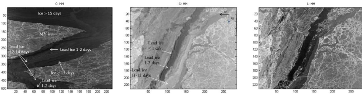
Figure 7 AIRSAR imagery from the Beaufort Sea. Left (scene 6830): Ice type labels overlaid C-band HH channel. Middle and right (scene 6832): Ice type labels overlaid C-band HH (middle). L-band HH (right).
