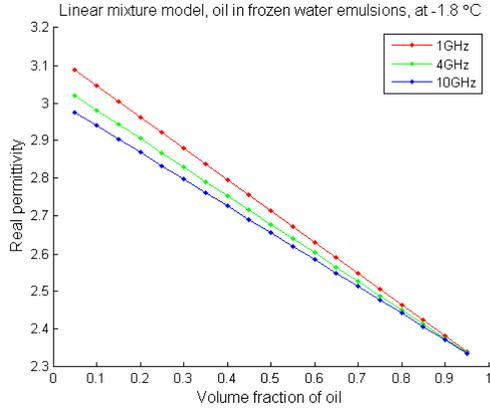
Figure 3 Real permittivity for oil emulsions in frozen water at  $-1.8^\circ\text{C}$ .
