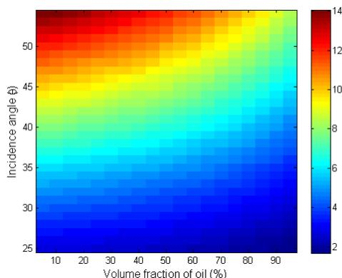
Figure 6 Co-polarization ratio as a function of  $\theta$  and oil volume fraction in sea ice mixture. Legend in dB.
