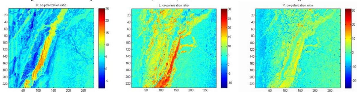
Figure 9 AIRSAR co-polarization ratios (VV/HH). C-, L- and P-band. Scene: 6832. Legends in dB.
