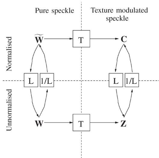
Fig. 1. Relations between the matrix representations introduced in the product model:  $\mathbf{Z} = T\mathbf{W}$ ;  $\mathbf{C} = T\tilde{\mathbf{W}}$  and by the normalizations:  $\mathbf{Z} = L\mathbf{C}$ ;  $\mathbf{W} = L\tilde{\mathbf{W}}$ .
